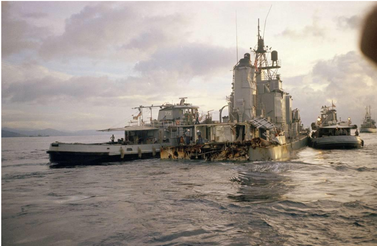
Sailors inspect damage to the U.S. Navy destroyer Frank E. Evans after it was cut in half in a collision with the light aircraft carrier Melbourne of the Royal Australian Navy in the South China Sea, 650 miles southwest of Manila, June 3, 1969. (AP)
